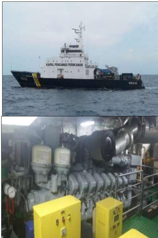
Fig. 1. The fishing control vessel Orca 02 and the ship's main propulsion.
