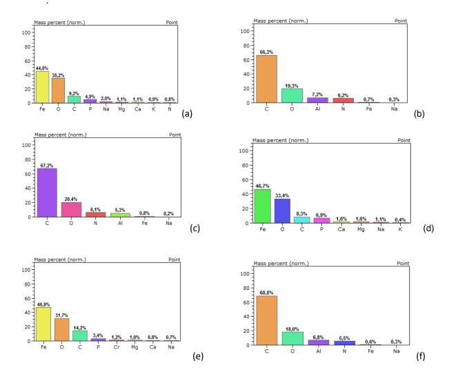
Figure 4: Chemical composition of electrodes EDS analysis, in the fifth day of experiment: (a) LI-V (b) LI- UV (c) BD-V (d) BD-UV (e) BT-V (f) BT-UV
