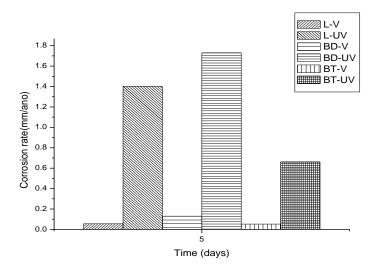
Figure 2: Corrosion rate for the three parts of the can in the fifth day of the experiment
