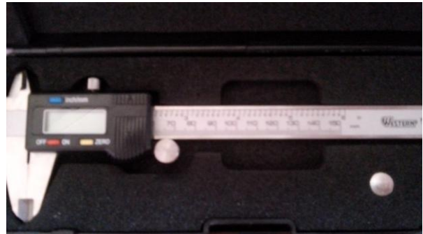
Figure 3. Sliding calliper rule, or pachymeter, used to measure size of injuries.
