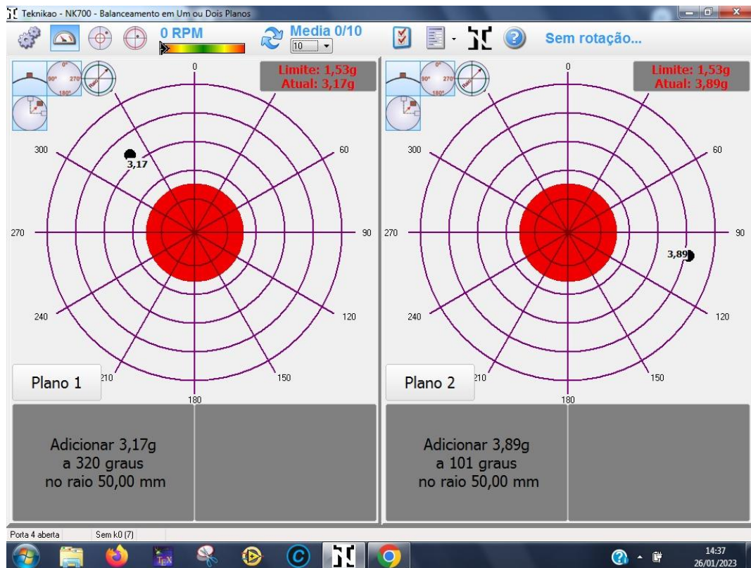
Figure 3: Teknikao software reports alert with the red color to the bad unbalance level. It means that the specimen is unbalanced, according with the grad of quality selected, 2023.
