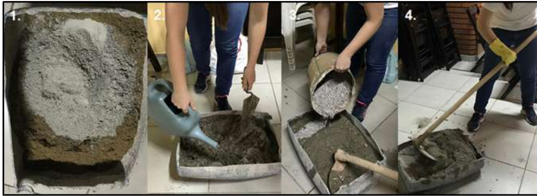
Figure 3. Mixing steps for manufacturing conventional concrete
