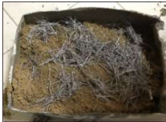
Figure 4 - Addition of fiber in concrete mix
