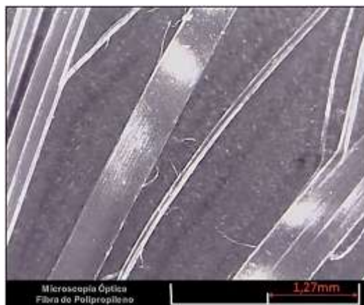
Figure 2 - FORTA FERRO® Polypropylene fiber optic microscopy
